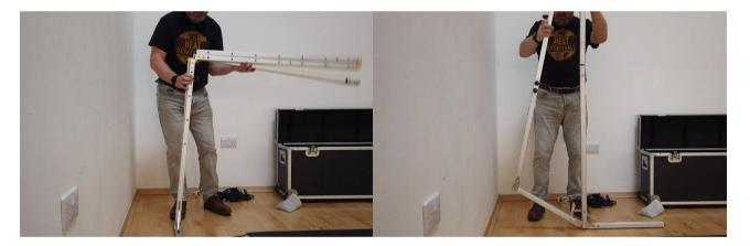
Unscrew a quarter turn the two bolts heads halfway down the back of the legs so that the top is free to slide up and down. – NOTE: only unscrew a quarter turn other wise there is a risk that the bolt heads will come away completely.
