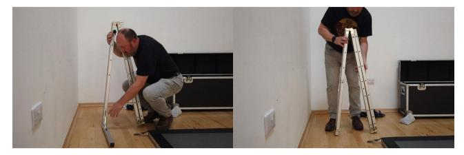
Take the back part of the leg with the two black bolt heads (opposite to the opened foot) and move it away from the foot so that it forms a triangle.
