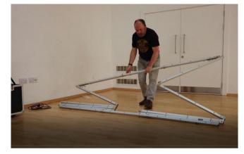
The joints of the frame can be gently straightened until they lock in place.
