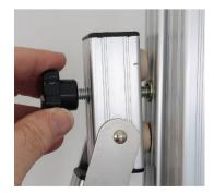
Retighten the two black head bolts on the back leg and make sure that the hinge locks are snapped into place at the bottom of the uprights.
