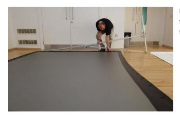
Locate the three screw in points on the screen frame and align the holes in the leg assembly. Screw a bolt through
